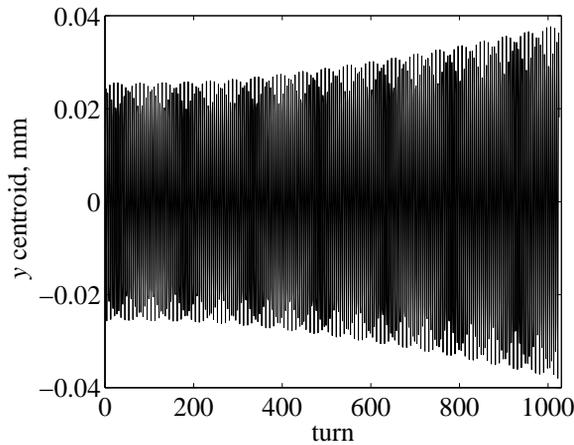
Figure 3: The vertical oscillation of the bunch centre.
