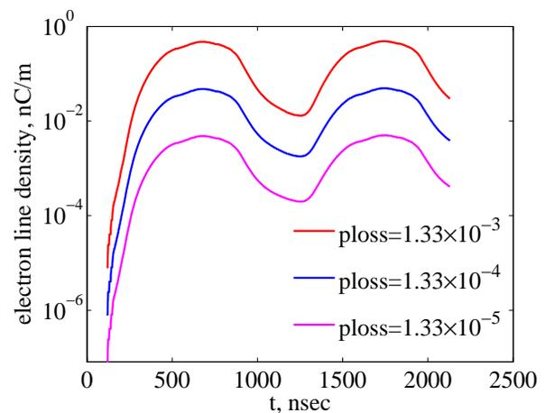
Figure 2: Electron line density for different proton loss.
