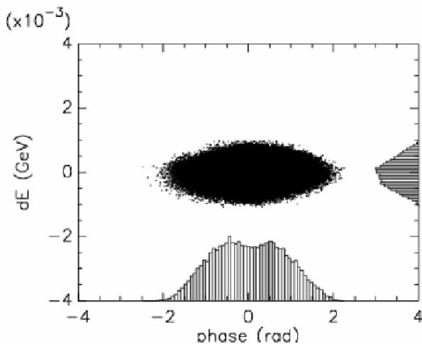
Figure 4: The longitudinal phase space distribution of the proton bunch.
