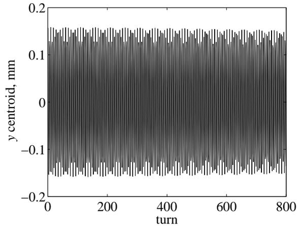
Figure 5: The vertical oscillation of the bunch centre.
