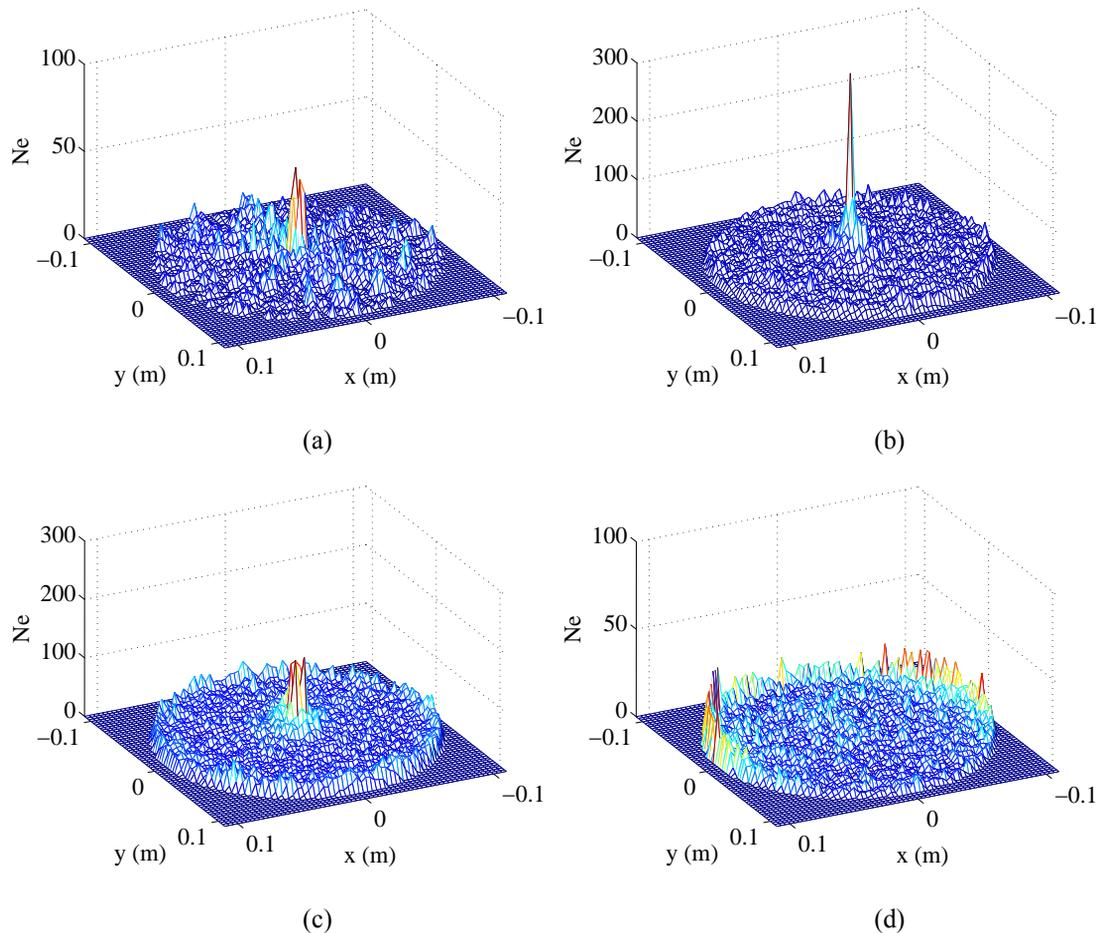
Figure 1: Electron distribution in the transverse section at the bunch head (a), bunch centre (b), peak of the electron density (c), and bunch tail (d).
