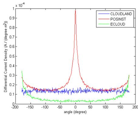
Figure 3: Azimuthal distribution in initial run. The primary photons strike the wall at zero degrees.
