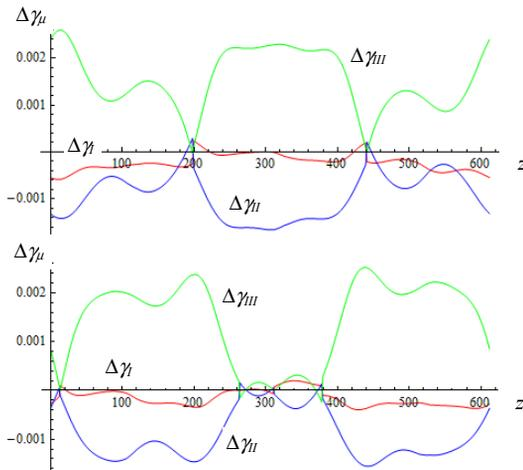
Figure 2: Change in cooling decrements vs. position of horizontal (top) and vertical (bottom) Be wedge of full angle 0.1rad.
