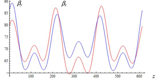
Figure 1:  $\beta$ -wave excited in “helical snake” due to difference in currents in solenoids of opposite polarity
