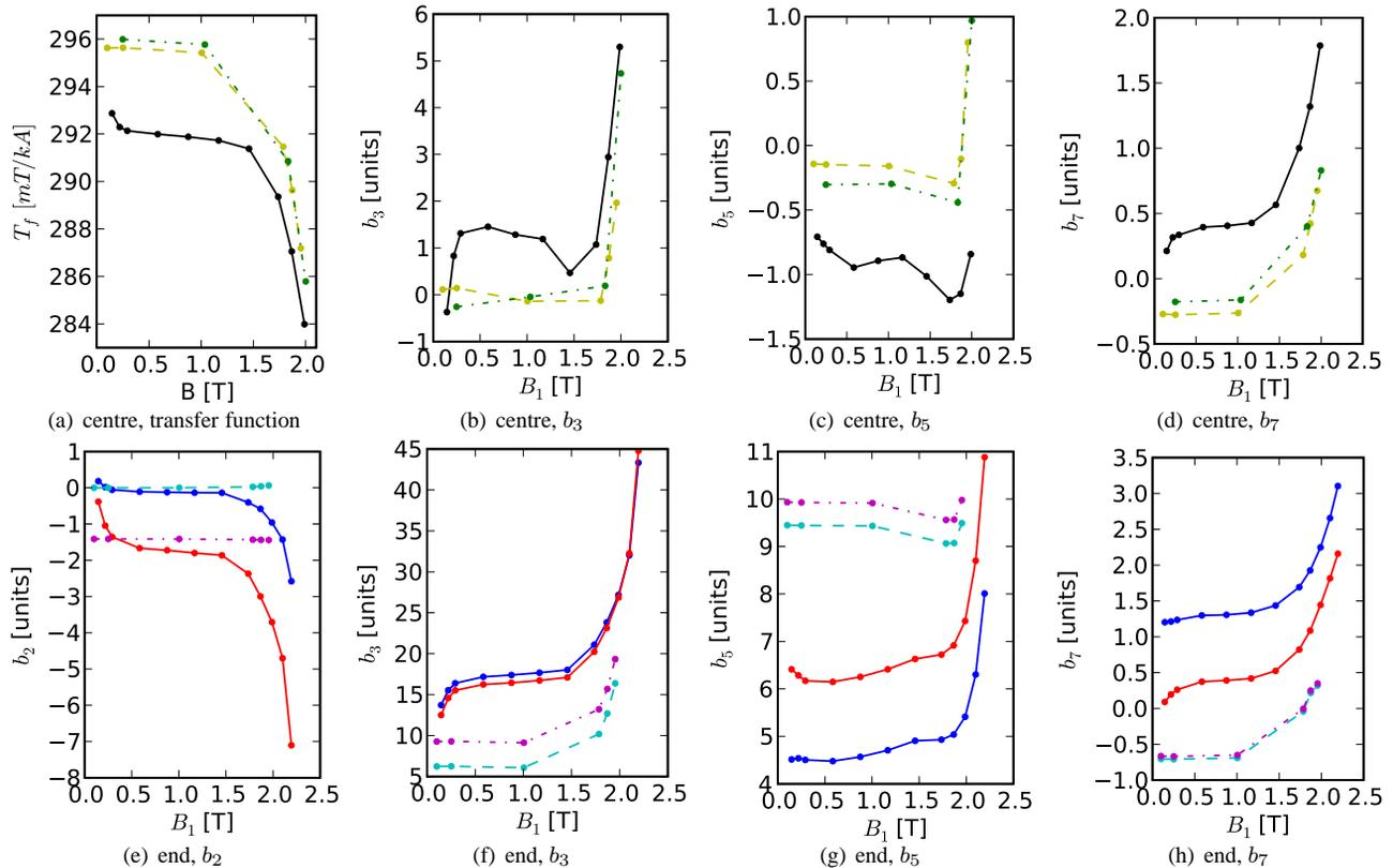
Figure 1: The measured (solid line) and calculated transfer function and harmonics versus the main field. centre: black – measured, yellow – TOSCA, green – ANSYS. end: connection side blue – measured, cyan – TOSCA; non connection side: red – measured, magenta – TOSCA.
