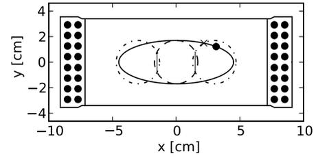
Figure 2: The gap of the measured magnet as well as the measurement positions of the coil probe. black filled circles — coil windings, dashed centre circle, dashed dotted circle  $x_m = \pm 3.0 \text{ cm}$ , coil probe measurement positions, solid line — ellipse used in reconstruction, dot on the ellipse – angle  $\psi_c$ , solid vertical lines – minimization lines.
