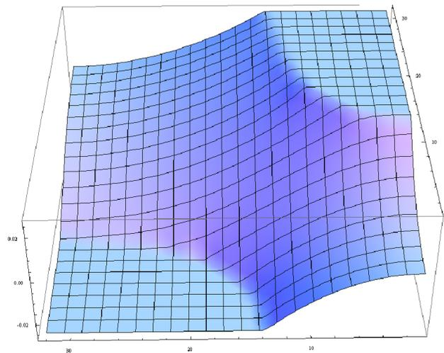
Figure 2: x-y-plane of the potential in a RFQ cell.
