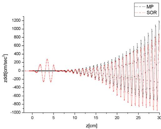
Figure 5: Acceleration based on electric field of particle with  $x=.1\text{cm}$  vs. longitudinal position for the low energy part of the RFQ.
