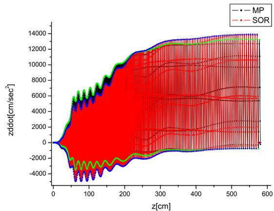
Figure 3: Acceleration based on electric field the synchronous particle sees vs. longitudinal position.
