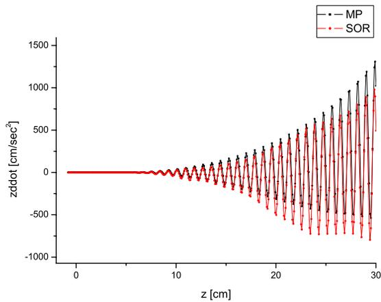
Figure 4: Acceleration based on electric field the synchronous particle sees vs. longitudinal position for the low energy part of the RFQ.
