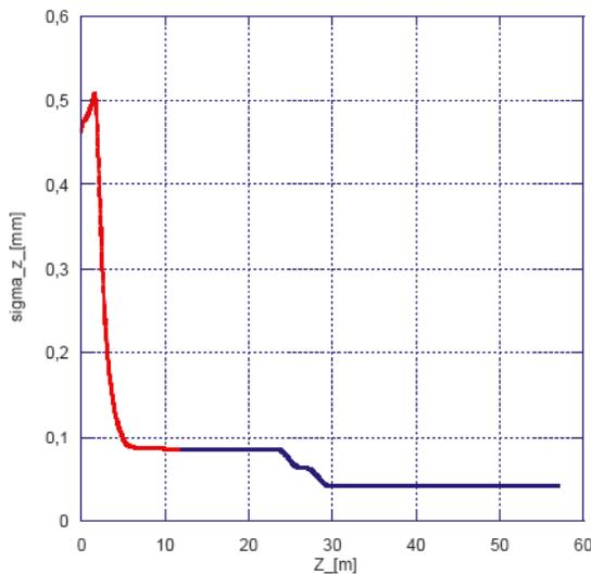
Figure 5: Rms length along the accelerator.
