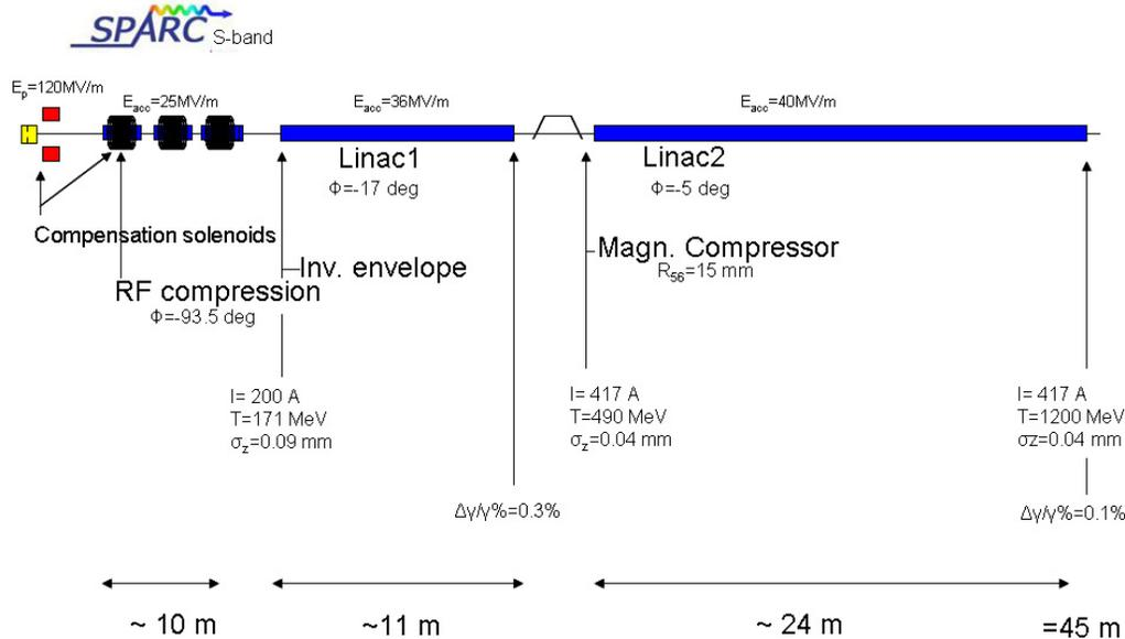
Figure 1: Schematic layout of the Sparc S-band photo-injector and C-band linac to 1.2 GeV.
