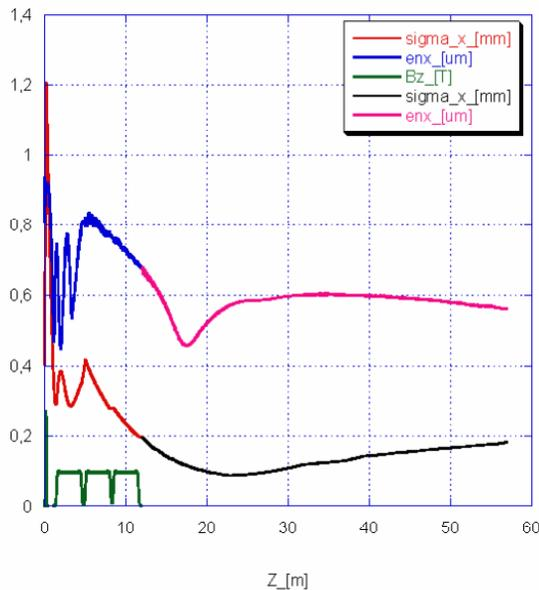
Figure 2: Emittance, rms spot size and the solenoid field along the accelerators up to 1.2 GeV. The different colour along the same line represents the S band (until about 12 m) and the C band
