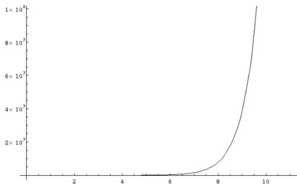
Figure 6: SASE output power along the undulator as predicted by Ming Xie scaling laws at 8 nm wavelength.
