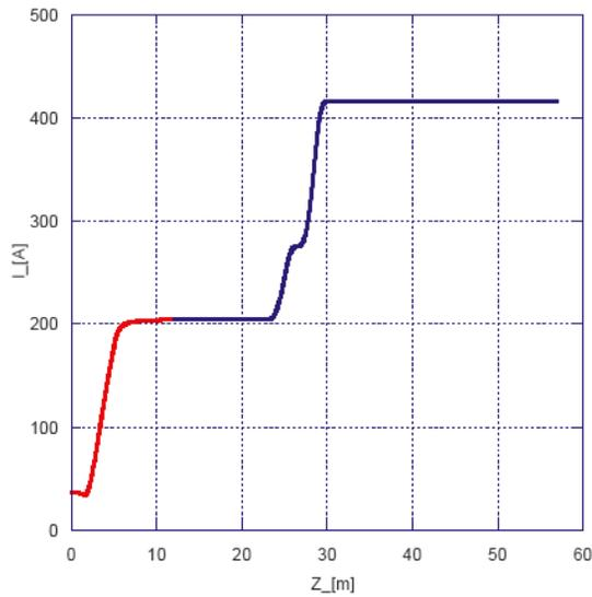
Figure 4: Current along the accelerator.
