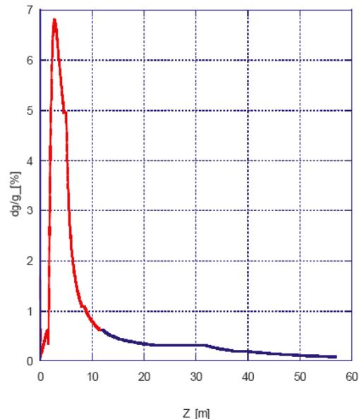
Figure 3: Energy spread along the accelerator.
