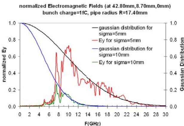
Figure 5: The spectra for different bunch sigma with beam pipe radius = 17.40 mm.
