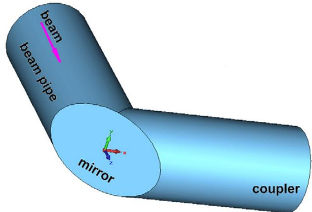
Figure 1: Structure for simulation of transition radiation using a moving Gaussian-distributed line charge.
