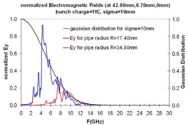
Figure 6: The spectra for different beam pipe sizes with bunch sigma = 10 mm.
