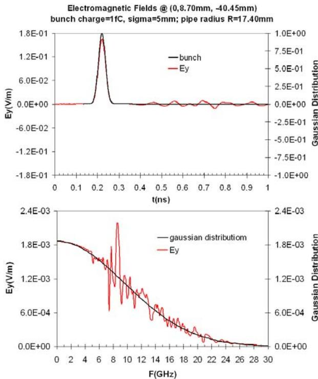
Figure 3: The electromagnetic field produced by a Gaussian bunch with 5-mm sigma. Top graph is the 2-D contour of  $E_x$  on the  $y=0$  plane at 0.2 ns. Middle graph shows  $E_y$  and the line charge density in the time domain, and in the frequency domain in the bottom graph. Data correspond to the point  $(x, y, z) = (0 \text{ mm}, 8.70 \text{ mm}, -40.45 \text{ mm})$ .
