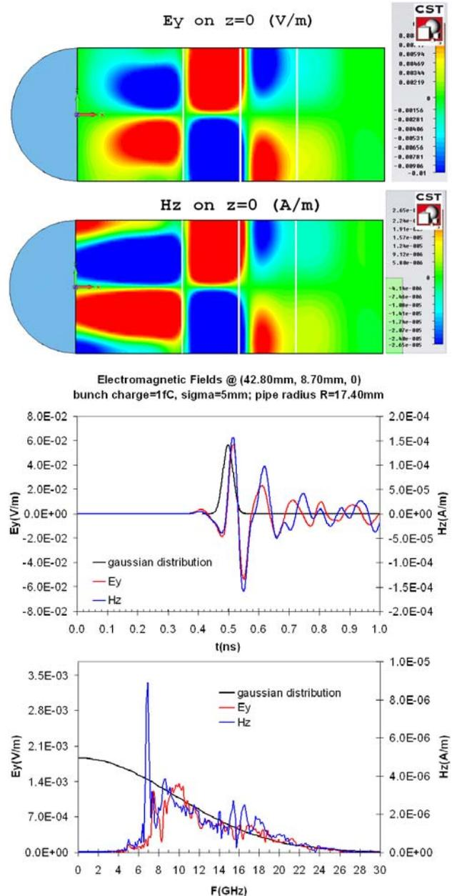
Figure 4: The electromagnetic field representing the transition radiation in the coupler. Top two graphs are the 2-D contours of  $E_y$  and  $H_z$  on the  $z=0$  plane at 0.5 ns. The third graph shows  $E_y$ ,  $H_z$ , and the assumed line charge at the light speed reflected by the mirror in the time domain, and in the frequency domain in the bottom graph. Data corresponds to the point  $(x, y, z) = (42.80 \text{ mm}, 8.70 \text{ mm}, 0 \text{ mm})$ .
