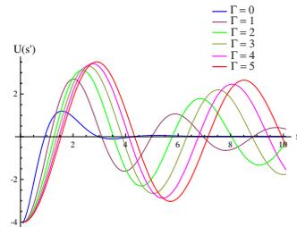
Figure 4: The longitudinal wake for various  $\Gamma$  values.
