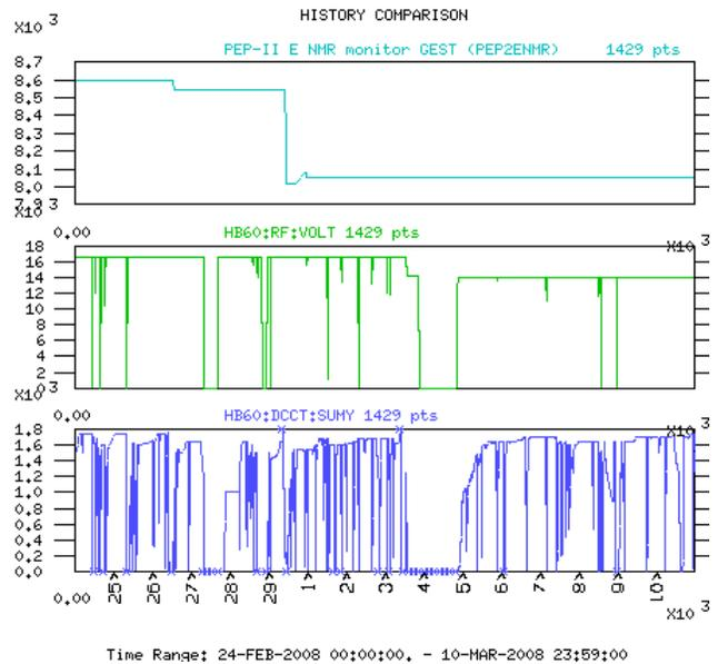
Figure 1: Energy, RF gap voltage and beam current during 3S to 2S transition. Energy (top plot) in MeV is calculated from HER magnet strengths. Middle plot shows the RF gap voltage remained at 16.5 MV until three days after the energy change. Bottom plot shows beam currents maintained at 1700 milli-amperes.
