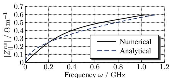
Figure 3: Low frequency range for longitudinal resistive wall coupling impedance ( $\sigma_w = 10^6$  S/m).
