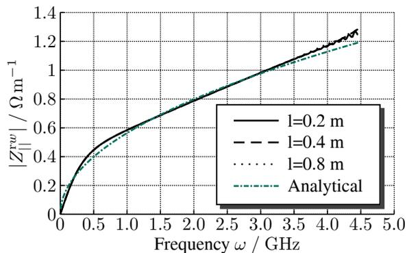
Figure 2: Longitudinal resistive wall coupling impedance for three model lengths: The result values have been normalized to 1 meter.
