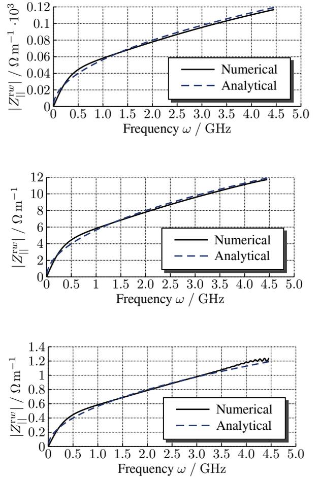
Figure 1: Longitudinal resistive wall coupling impedance for a pipe with circular cross-section, calculated for three different conductivities: 100, 10000 and 1000000 S/m (from top to bottom)
