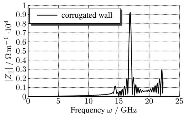
Figure 4: Longitudinal coupling impedance for corrugated wall (diameter 10 cm, corrugation period 6 mm, corrugation amplitude 4 mm).
