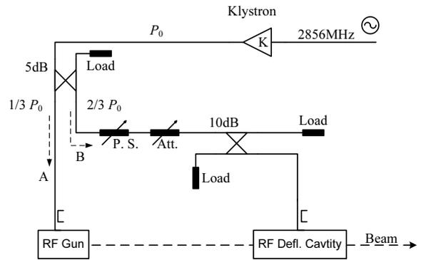
Figure 2: The power feeding scheme for TTX Phase-I
