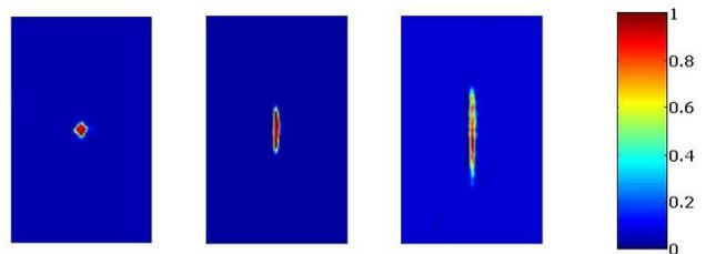
Figure 4: Beam spot with different deflection (attenuation from left:  $>30\text{dB}$ ,  $15\text{dB}$ ,  $7\text{dB}$ )
