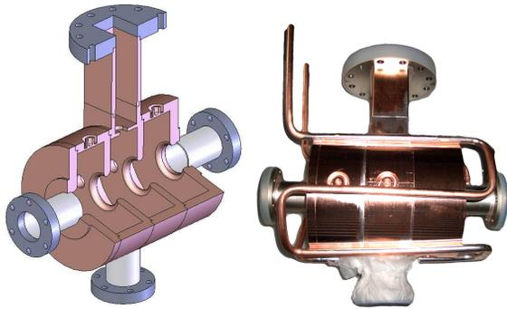
Figure 1: The CAD model and a photo of the deflecting cavity
