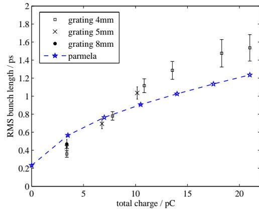
Figure 7: The bunch length with respect to the bunch charge (measured and comparison with Parmela)
