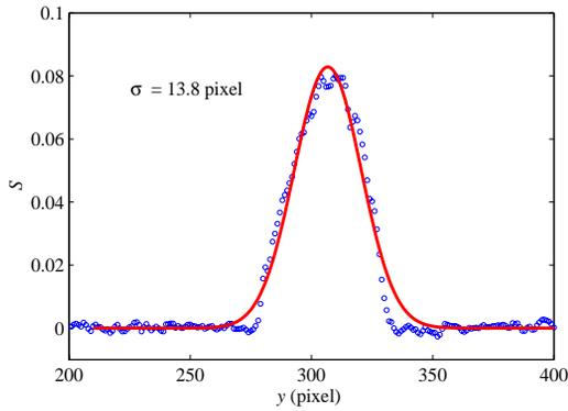
Figure 5: Gaussian fit of the bunch profile at screen
