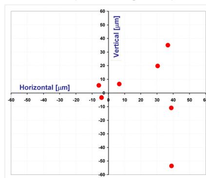
Figure 4: Mechanical offset of assembled BPM blocks. Data obtained from 3D coordinate measurement machine.
