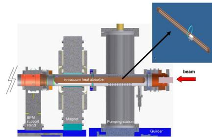
Figure 1: 3D model of the in-vacuum heat absorber used to prevent synchrotron light from hitting the vacuum chamber downstream the dipole magnet.
