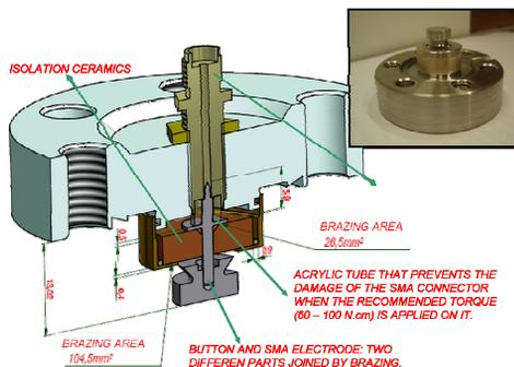
Figure 3: 3D model of the button and a picture of the button after all brazing processes.
