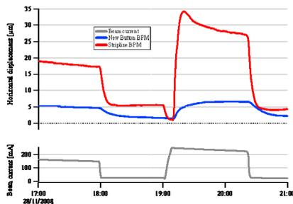
Figure 6: The horizontal drift of the new BPMs is almost one order of magnitude smaller than in the stripline BPMs.
