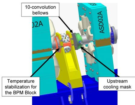
Figure 7: 3D model of the new BPM in the storage ring.
