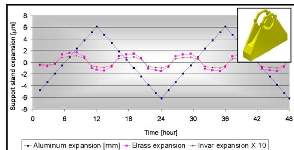
Figure 2: Simulation of the support stand thermal performance.
