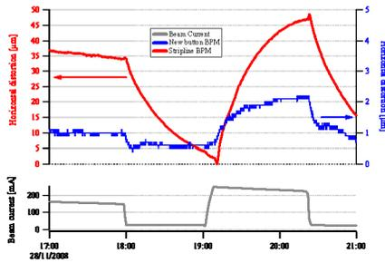
Figure 5: The horizontal distortion (uneven expansion) is more than one order of magnitude smaller in the new button BPMs.
