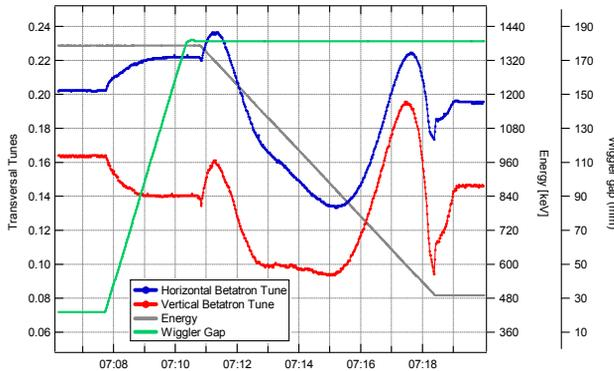
Figure 5: Betatron tune log during a wiggler movement.
