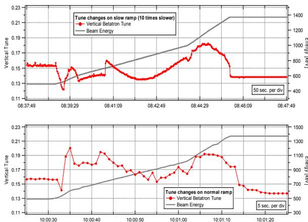
Figure 6: Vertical betatron tune along slow (up) and normal (down) ramps.
