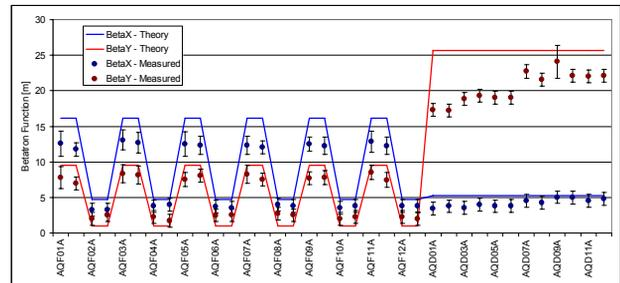
Figure 3: TuneLogger’s betatron function measurement.
