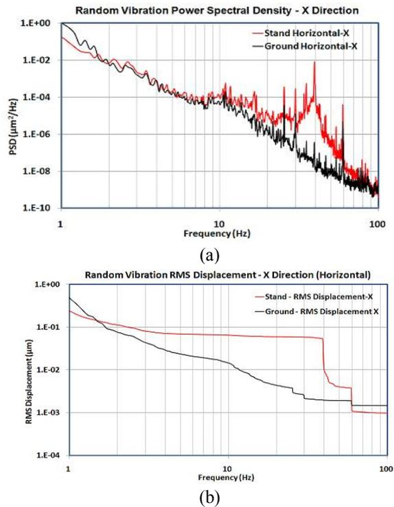
Figure 5: (a) Power spectral density and (b) RMS displacement plots for horizontal vibration.
