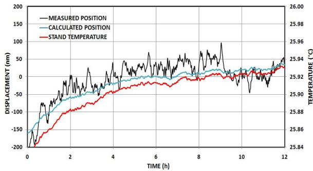
Figure 4: Plot of positional data from laser interferometer.
