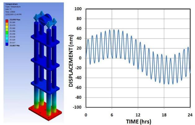
Figure 2: Temperature distribution (left) and plot of vertical deformation.
