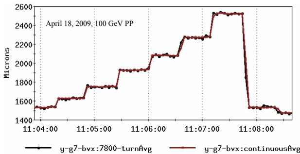
Figure 6: 7800-turn average orbit vs. continuous average orbit (divide value =  $2^{13}$ ) during beam position scan.
