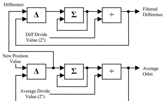
Figure 7: BPM continuous average orbit and filtered difference signal.
