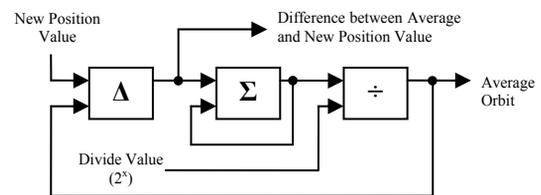
Figure 1: RHIC BPM continuous average orbit algorithm.
