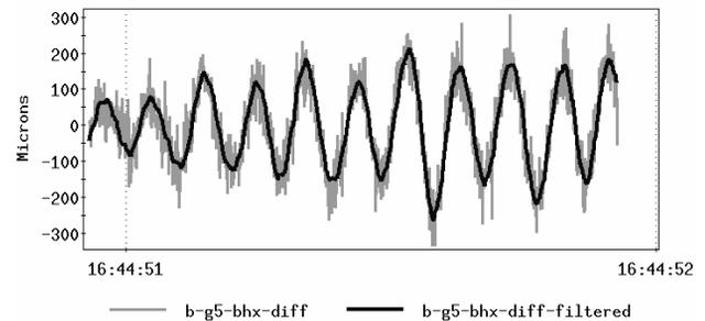
Figure 8: BPM Raw Difference vs. Filtered Difference.
