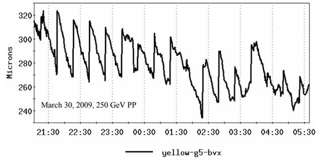
Figure 4: Continuous average orbit for a single BPM during an 8 hour RHIC store.
