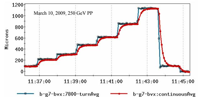
Figure 5: 7800-turn average orbit vs. continuous average orbit (divide value =  $2^{16}$ ) during beam position scan.
