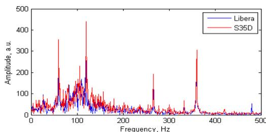
Figure 1: Overlaid spectra of beam motion in the horizontal plane. The data are from both Libera Brilliance and FPGA based receiver.
