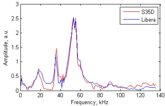
Figure 8: Spectra of the vertical oscillations caused by the injection transient. 54 kHz line corresponds to the vertical betatron oscillations.
