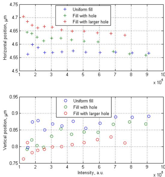
Figure 10: Beam position measured by Libera Brilliance vs. intensity for different fills.
