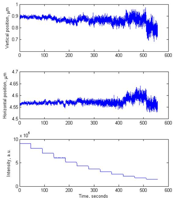
Figure 9: Time dependence of Y, X and Sum signals while the uniform beam is being steered in the horizontal plane.
