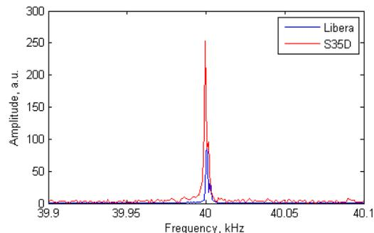
Figure 3: Quadrupole power supplies noise line observed by two BPM receivers (Libera Brilliance and FPGA based receiver).
