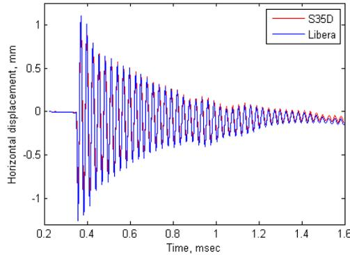
Figure 5: Horizontal transient caused by the injection kickers. There is a remarkable agreement in the two curves except only small offset are observed towards the end of the transient.
