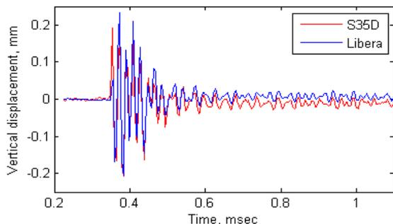
Figure 7: Vertical transient caused by injection kickers.
