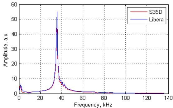
Figure 6: Spectra of horizontal beam motion excited by the injection transient. The strong line at 35.6 kHz corresponds to the horizontal betatron frequency and synchrotron oscillations manifest themselves as a small peak at low frequency.
