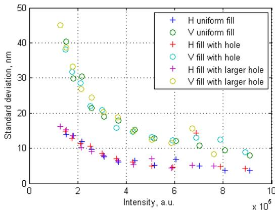
Figure 11: Libera Brilliance beam position measurement noise dependence on intensity for different fills.
