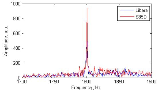
Figure 2: Synchrotron motion line observed by two BPM receivers (Libera Brilliance and FPGA based receiver).
