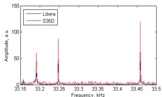
Figure 4: Details of horizontal beam motion in 30 kHz region observed by two BPM receivers (Libera Brilliance and FPGA based).
