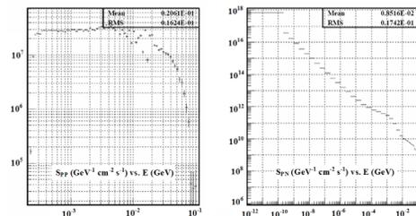
Figure 8: Estimated proton and neutron energy spectra.
