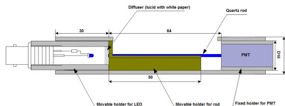
Figure 9: SiO<sub>2</sub> fiber transmittance evaluation set-up.
