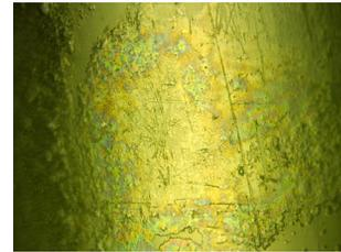
Figure 13: Crystal surface damage and fragment tracks.
