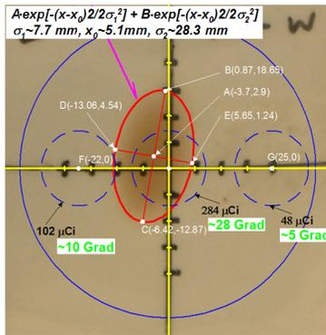
Figure 5: Beam profile and measured peak dose.
