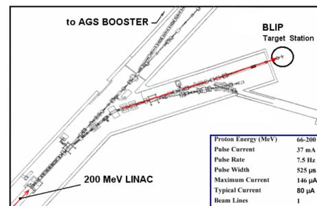
Figure 3: Schematic of the BNL BLIP irradiation facility.
