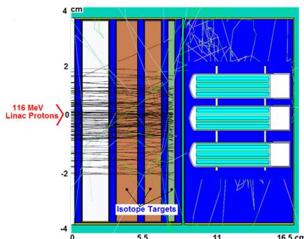
Figure 6: Particle tracks generated by the MARS15 code.
