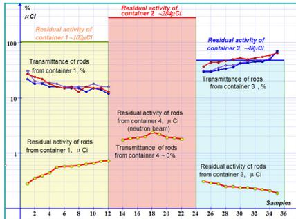
Figure 10: Transmittance of irradiated SiO<sub>2</sub> fibers.
