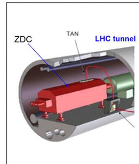
Figure 1: Configuration of ZDC Calorimeter in LHC.
