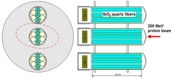
Figure 4: Fiber arrangement for the 200 MeV irradiation.
