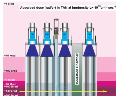
Figure 2: ZDC layout and anticipated dose in SiO<sub>2</sub> fibers.
