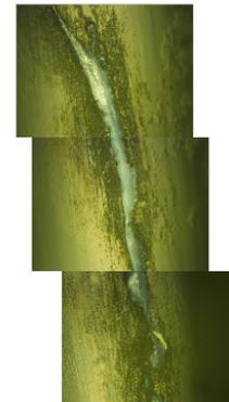
Figure 15: Fragment track and damage on crystal surface.
