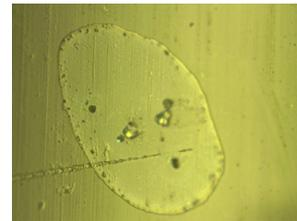
Figure 14: Thermal spike on the fiber surface.
