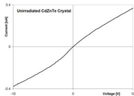
Figure 9: Un-irradiated CZT crystal  $I-V$  characteristic.
