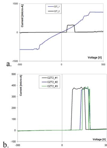
Figure 10:  $I-V$  characteristic of irradiated CZT crystal.
