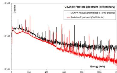
Figure 12: “Preliminary” comparison of photon spectra between irradiation test and MCNPX simulation.
