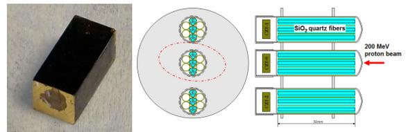
Figure 2: CdZnTe bar detector and irradiation configuration under 200 MeV proton beam.
