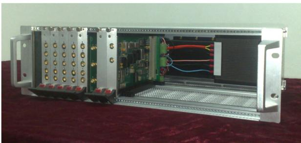
Figure 6: The phase monitor system for CRM cyclotron.
