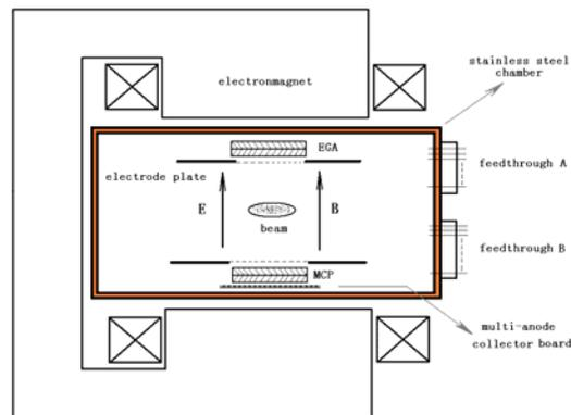
Figure 1: Horizontal IPM detector frame of CSNS-RCS.
