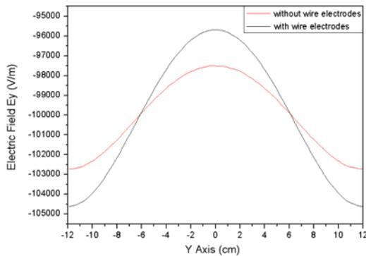
Figure 4: Calculated  $E_y$  amplitude for the edge before and after wire electrodes were added.
