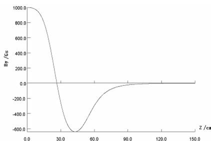
Figure 7: Magnetic field  $B_y(0)$  distribution along z axis, integral value is zero.
