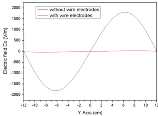
Figure 3: Calculated  $E_x$  amplitude versus y position for one edge before and after wire electrodes were added.
