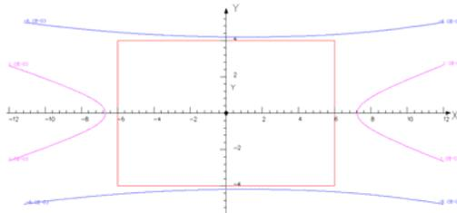
Figure 6: Relative deviation of  $B_y$  from  $B_y(0)$  on central plane.
