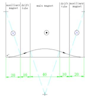
Figure 5: Schematic diagram of IPM magnets.
