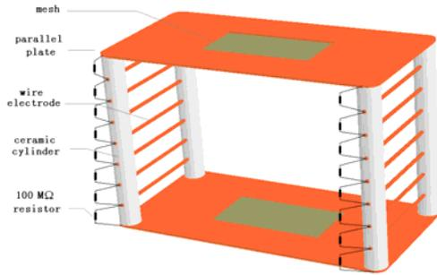
Figure 2: Schematic diagram of electric field system for IPM of CSNS-RCS.
