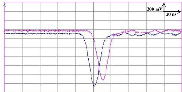
Figure 3: Visualisation of  $\Sigma$  signals of two BPMs.
