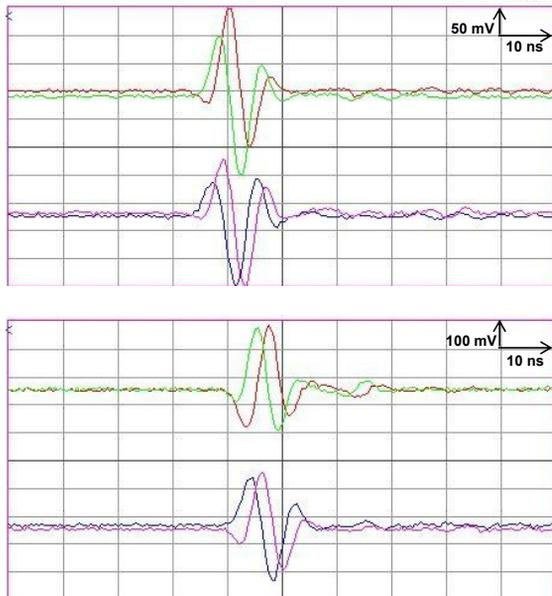
Figure 4: Visualisation of I and Q signals of two BPMs in vertical and horizontal frame in “10 bunches mode”.
