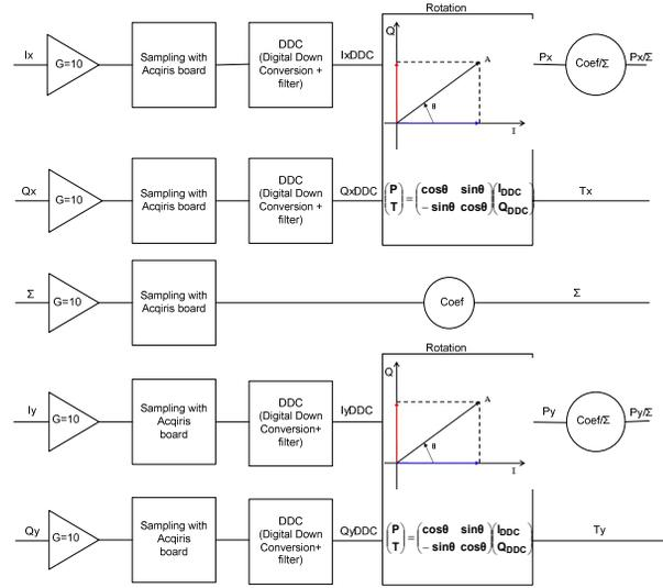
Figure 2: Schematic of signal post-processing.
