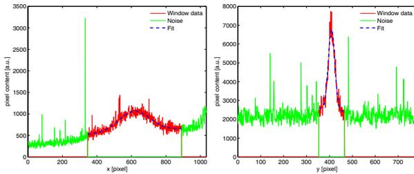
Figure 4: Example of an analyzed horizontal (left) and vertical (right) beam profile. The green line is signal outside the ROI, the red line is the part of the signal used for the analysis and the blue curve is the Gaussian fit to estimate the rms beam size.
