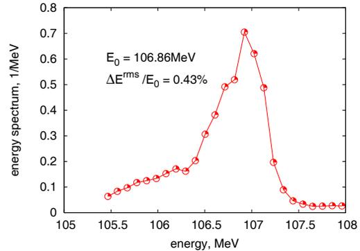
Figure 3: Energy spectrum for a 3.7 nC beam in MBM.
