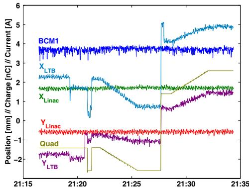
Figure 2: Positions at the Linac and LTB BPMs during the quadrupole scans. The rms stability (inferred from data taken during the first two minutes) is:  $\Delta_{x,y-Linac}^{rms} = (65, 71)\mu\text{m}$ ;  $\Delta_{x,y-LTB}^{rms} = (59, 72)\mu\text{m}$ .
