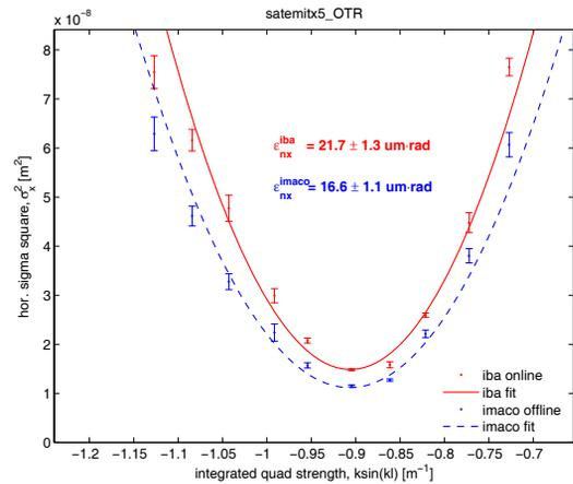
Figure 5: Example of an emittance measurement in the horizontal plane in MBM using the OTR screen ( $Q=3.8$  nC).
