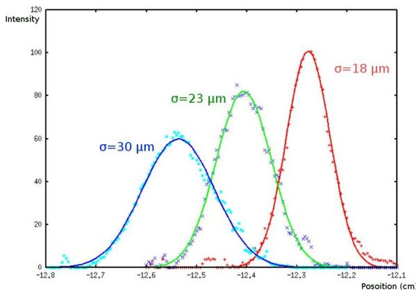
Figure 4: Variation of beam size for betasing 1 settings
