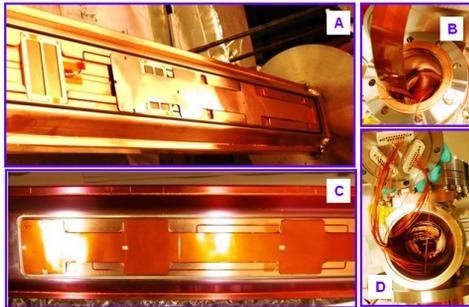
Figure 8. (A) Flexible circuit through duck-under channel, with (B) soldering pad end at RFA connection port. (C) After attaching all connection leads, the circuit was precisely located on top of the grids frames by five ceramic head pins. (D) All 45 leads connected to three 15-pin D-type feedthroughs on a 4-5/8” flange.
