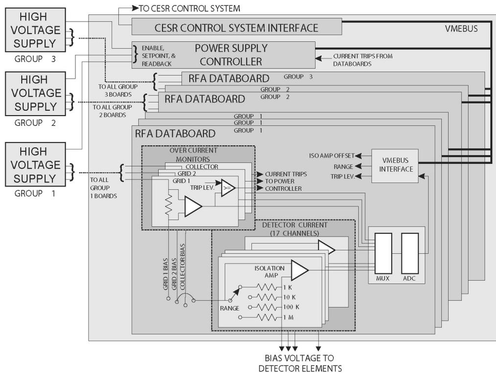
Figure 2: Schematic showing the high voltage power supply system and the RFA current monitor boards.
