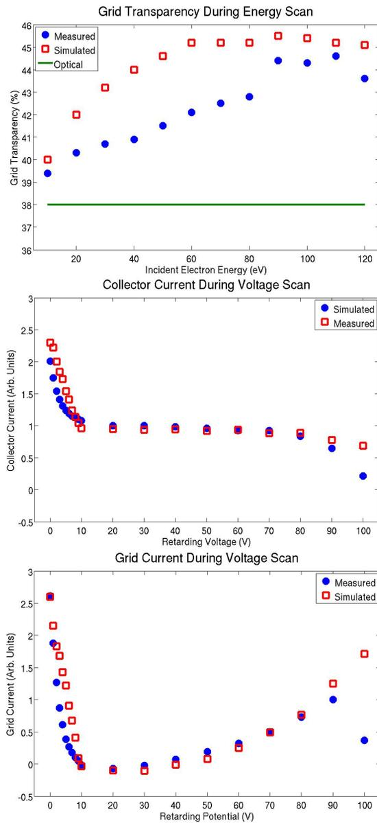
Figure 3: Plots showing electron gun studies of the performance of the thin RFA structure with a front plate with holes matching the wiggler vacuum chamber specifications. The top plot shows the fraction of electrons reaching the collector versus the energy of the incident electrons. The bottom pair of plots show the collector and grid currents observed during a retarding voltage scan with 110eV incident electrons.
