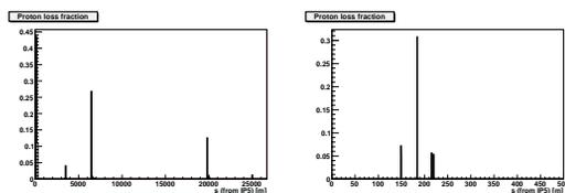
Figure 2: The loss distribution of IP protons for a multi-turn simulation, showing the loss fraction of the protons as a function of distance around the LHC ring for the whole ring (left-hand plot) and the LSS5 region (right-hand plot).
