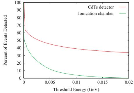
Figure 4: Percent of event detected versus the threshold energy.
