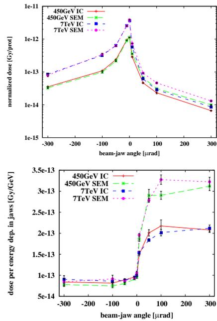
Figure 4: Top: Normalized BLM signal is plotted for a TCP collimator versus beam-jaw angle between  $\pm 300 \mu\text{rad}$ . Bottom: Ratio of BLM signal to total energy deposition in the jaws is plotted for a TCP collimator versus beam-jaw angle.
