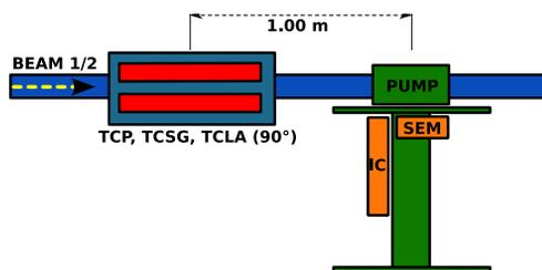
Figure 1: Side view of a “collimator-detector cell” composed of a collimator, an IC, and a SEM, as installed in the LHC cleaning insertions. A vertical collimator is shown.
