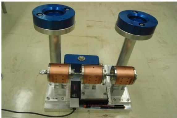
Figure 3: PBPM triplet for resolution measurement.
