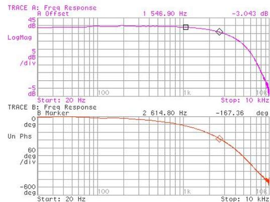
Figure 5: The frequency response of the LPF. The measured gain is 39 dB and the 3 dB point of the filter is 2.6 kHz which is close to the SPICE model calculation.
