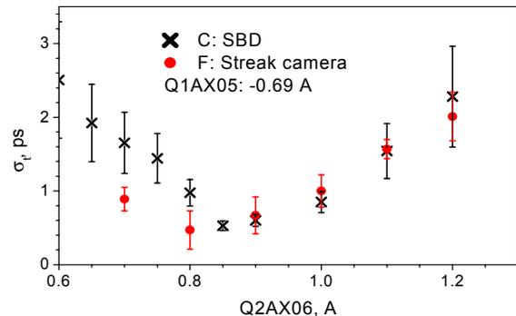
Figure 6: The bunch  $\sigma_t$  obtained with the parametric presentation via the SBD signal and directly measured with a streak camera vs. the quadrupoles settings.
