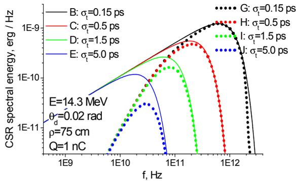
Figure 2: Computed CSR spectral energy vs.  $\sigma_t$  for 1 nC bunch emitted in the A0 Photoinjector dipole magnet (solid lines), and convolved with the SBD response characteristic (dotted lines).
