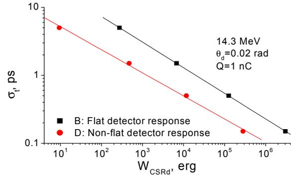
Figure 3: The bunch duration  $\sigma_t$  as a function of the CSR energy detected in a latitudinal angle of  $\pm 20$  mrad.
