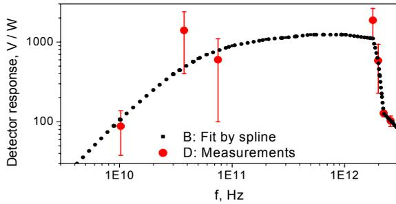
Figure 1: Quasi-optical SBD evaluated and measured response.
