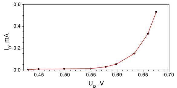
Figure 4: The SBD I-V characteristic.
