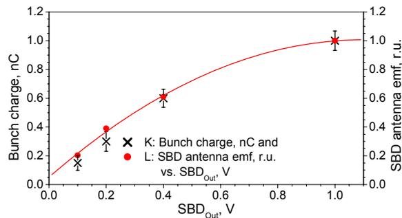
Figure 5: Measured dependence of the bunch charge (left scale) and computed dependence of the SBD antenna emf (right scale) on the detector output signal.
