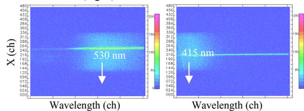
Figure 3: Imaging spectrometer results using the CCD camera readout in x- $\lambda$  space for YAG:Ce crystal plus an Al mirror (left) and the LSO:Ce crystal plus an Al mirror (right). The localized x extent of the COTR streak in wavelength is evident in both cases.
