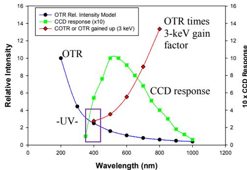
Figure 5: Analytical representations of the OTR dependence on  $1/\lambda^2$  and OTR times the 3-keV gain factor, or COTR. The CCD camera response is also shown.
