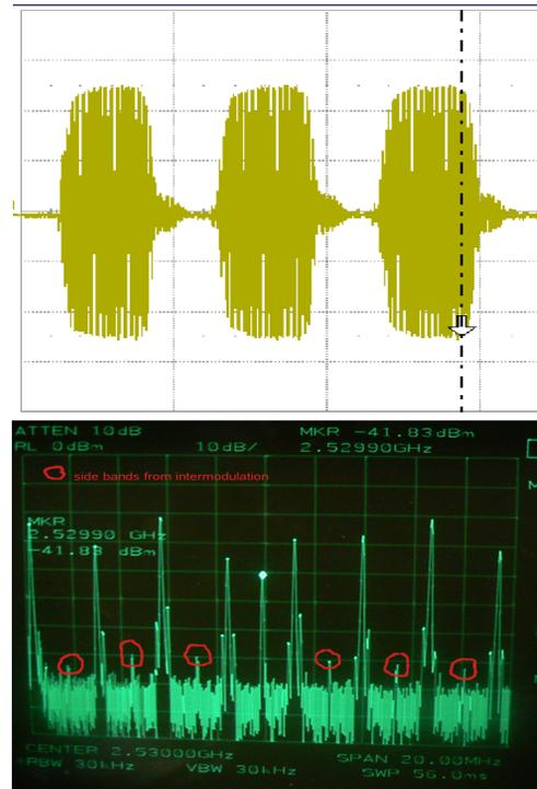
Figure 5: Signal generated to resemble fill pattern of beam, and demonstration of sidebands produced purely from inter modulation
