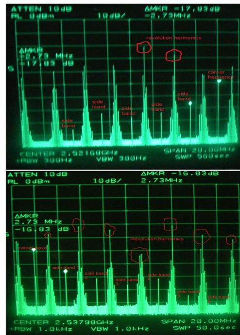
Figure 2: Left and right sidebands with carrier signal in the presence of beam
