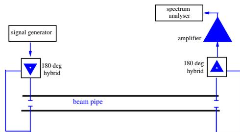
Figure 4: Schematic of the layout of the experiment
