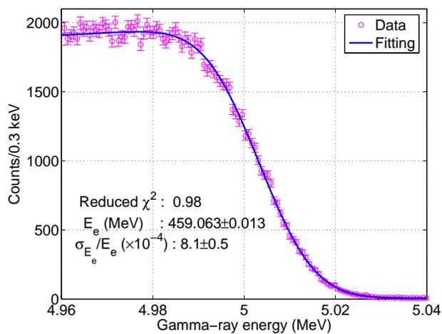
Figure 4: Illustration of the fitting on the high energy edge of the measured gamma beam spectrum. The goodness-of-fit is given by the reduced  $\chi^2$ . The determined electron beam energy  $E_e$  and relative energy spread  $\sigma_{E_e}/E_e$  as well as the overall uncertainties associated with them are also shown.
