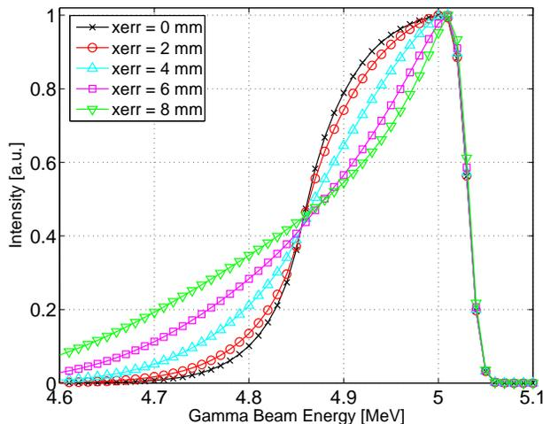
Figure 1: The energy spectrum of gamma-ray beam produced by Compton scattering of a 460 MeV electron beam with a 790 nm laser beam. The gamma beam is collimated by a collimator with radius of 12.7 mm placed 60 m downstream of the collision point. The spectrum is calculated for different alignment of the collimator from 0.0 mm to 8.0 mm in the horizontal direction.
