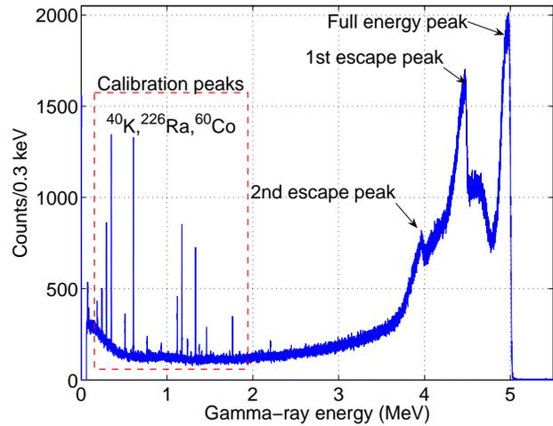
Figure 3: A typical HI $\gamma$ S beam spectrum measured by a large volume 123% efficiency HPGe detector. The radiation sources of  $^{226}\text{Ra}$  and  $^{60}\text{Co}$  as well as the nature background from  $^{40}\text{K}$  are used in the real time for the detector energy calibration.
