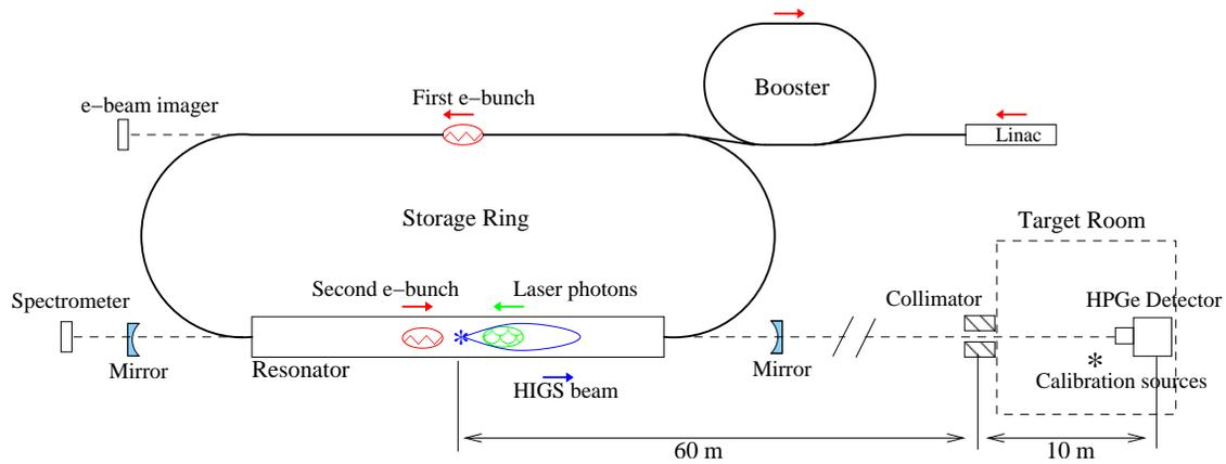
Figure 2: Schematic of the HI $\gamma$ S beam production and measurement at Duke University.
