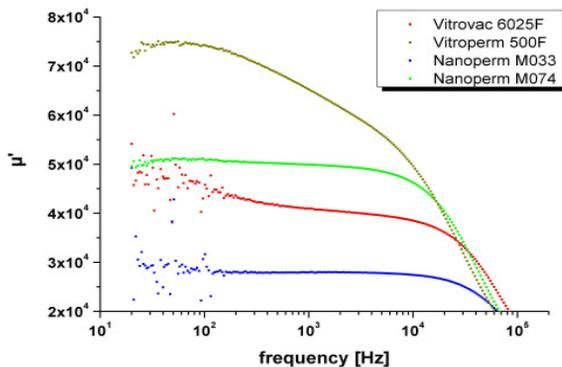
Figure 3: Real part  $\mu'$  of the relative permeability of different nanocrystalline samples of Vitroperm and Nanoperm at 4.2 K.
