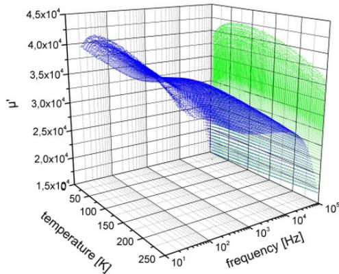
Figure 2: Real part  $\mu'$  of the relative permeability of Nanoperm M033 (50 windings) in the temperature range between 4.2 and 250 K.
