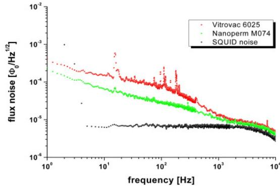
Figure 6: Measured noise contribution of amorphous Vitrovac 6025 and nanocrystalline Nanoperm M074.
