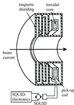
Figure 1: Simplified schematic view of the magnetic shielding, the toroidal pick-up coil, and the SQUID.
