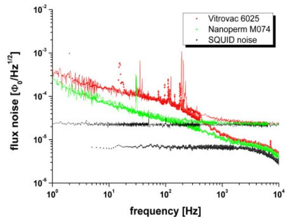
Figure 5: Spectral flux noise density of Vitrovac 6025 and Nanoperm M074 toroidal cores generated by one superconducting turn connected across the SQUID input coil. The black curves show the intrinsic noise of the SQUID using two different electronics (see text for details).
