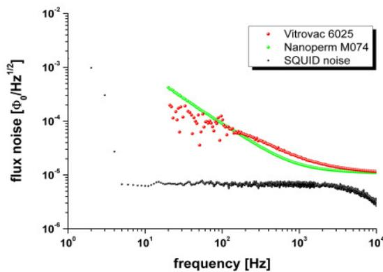
Figure 7: Calculated 1/f magnetization noise of Vitrovac 6025 and Nanoperm M074 using the Fluctuation-Dissipation Theorem.
