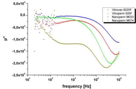
Figure 4: Imaginary part  $\mu''$  of the relative permeability of different nanocrystalline samples of Vitroperm and Nanoperm at 4.2 K.
