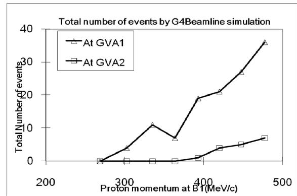
Figure 5: Relative number of expected proton counts in GVA1 and GVA2 counters as a function of the proton momentum at the entrance of the first dipole.
