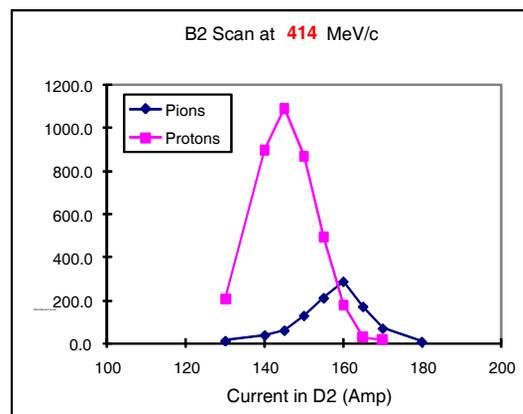
Figure 3: Relative protons and pions rate as a function of the current in the second dipole (D2) for a momentum selected in D1 equal to 414 MeV/c.
