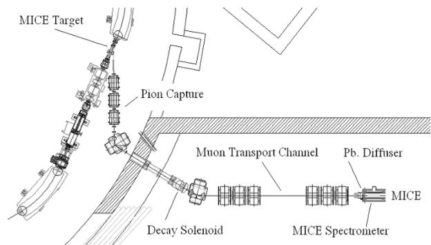
Figure 1: Schematic of the MICE beam line at ISIS, Rutherford Appleton Laboratory, UK.
