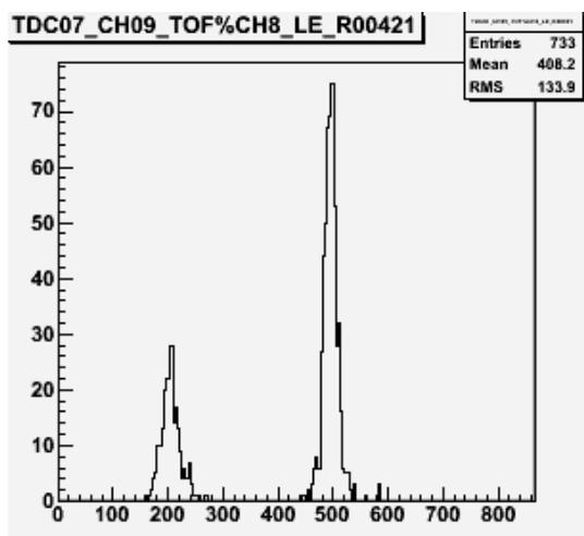
Figure 2: The first spectrum of the time of flight between GVA1 and GVA2 as it's available from the MICE online monitoring.
