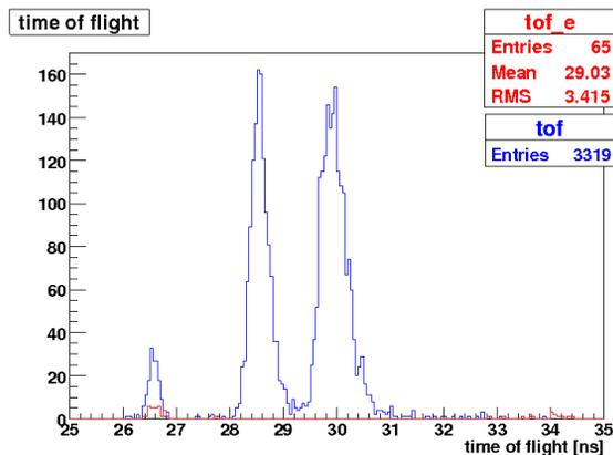
Figure 4: Time of Flight spectrum between TOF0 and TOF1 after calibration and time walk corrections. The red spectrum is obtained with the positron beam at 100 MeV/c. It is used to fix the horizontal scale. The blue spectrum is obtained at 300 MeV/c. The positron, muon and pion components are clearly separated.
