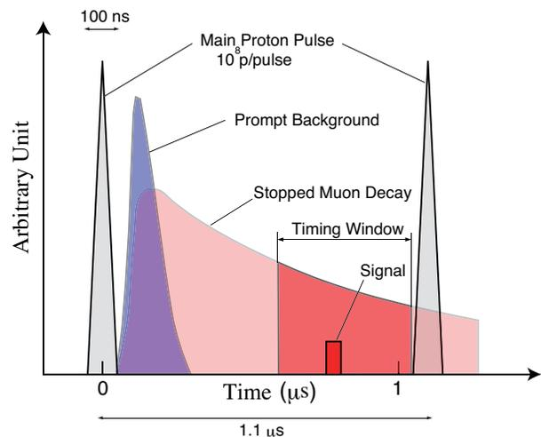
Figure 2: Required timing structure for the COMET experiment.
