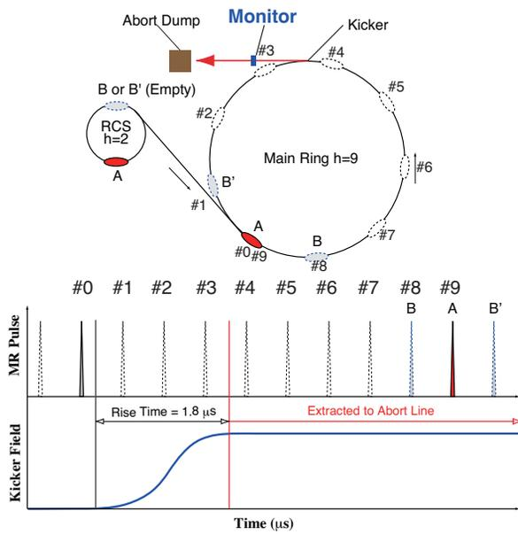
Figure 3: Fast extraction method.
