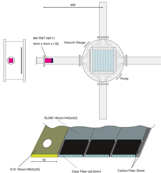
Figure 4: Beam monitor for abort line measurement.
