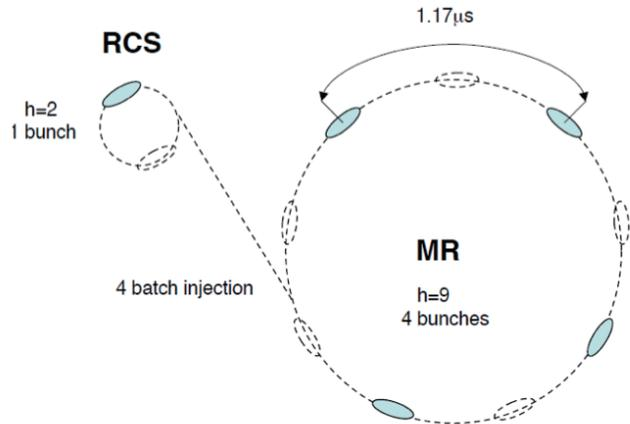
Figure 1: Simplest scheme of MR Injection for COMET experiment.
