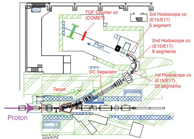
Figure 6: Beam line layout for secondary beam methods at Hadron experimental hall.
