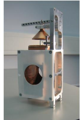
(b) A photograph of the detector, shown in its mechanical assembly. The magnet is not shown in this picture.
