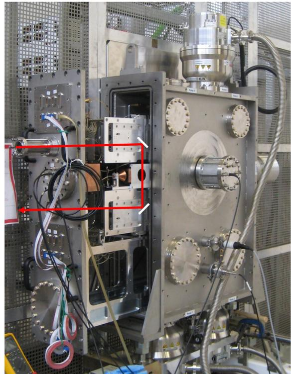
Figure 1: The vacuum vessel and the components required to make the beam density distribution measurement. In the centre of the picture the detector's copper Faraday cup can be seen. The central position of the mirrors is shown schematically in white, with the corresponding laser path in red.
