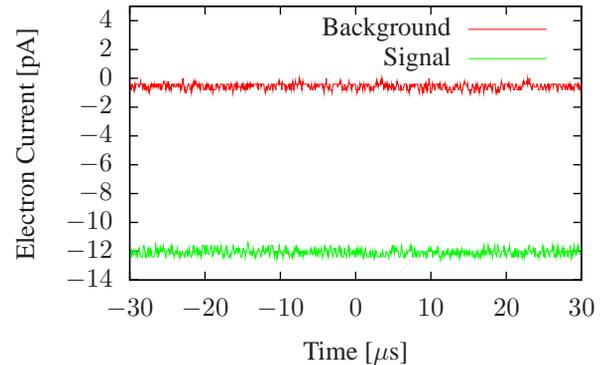
Figure 5: An oscilloscope trace showing that electrons are being detected when the filament is on (signal) and not when it is off (background).
