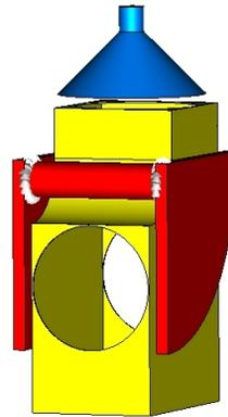
(a) A schematic of the detector. The magnet is shown in red, the accelerating sheath in yellow and the Faraday cup in blue.
