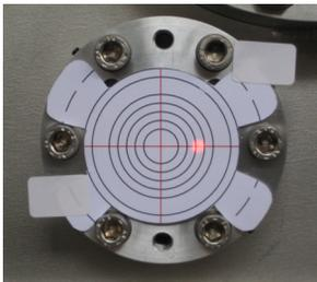
(b) A target mounted on the output window. The target's radii are 5 mm, 7.5 mm, 10 mm and so on. The movable stages are nearest to the vessel wall that the windows are mounted in (i.e. this is the configuration with the shortest path length).
