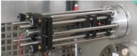
(a) The alignment laser jig, mounted on the laser input window. The output window is positioned 220 mm below the input window.
