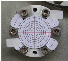
(c) For this picture the stages were moved to the furthest position from the vessel wall with the windows mounted in (such that the extra path length is 400 mm). Note that the spot has moved by  $\sim 7$  mm, compared to its position in Figure 2b.
