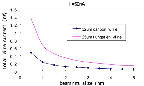
Figure 6: Max. total wire currents vs. beam RMS sizes.
