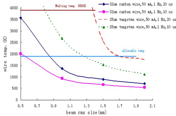
Figure 3: Max. wire temperatures vs. beam RMS sizes.
