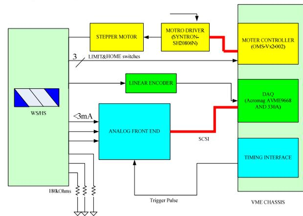
Figure 7: Block diagram of the electronic system for WS/HS.
