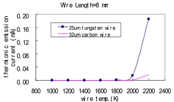
Figure 5: Thermionic currents vs. wire temperatures.
