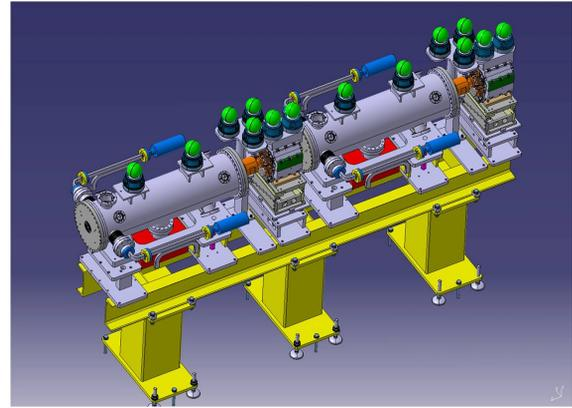
Figure 1: 3D view of a TBL cell with the PETS tanks, the BPS's and the quadrupoles.
