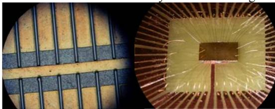
Figure 5: A magnified view showing few pixels of the photoconductive IR array detector (left). The interface board and the array detector showing the connection among pixels and the interface board made by gold bonding wires (right).
