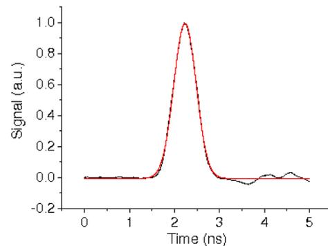
Figure 4: The shape of a typical  $e^+$  bunch (black curve) and its Gaussian fit (red curve) at IR wavelengths.
