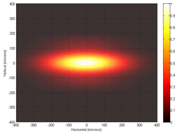
Figure 2: Simulated distribution of the IR photon beam at 10  $\mu\text{m}$  as obtained by the SRW software.
