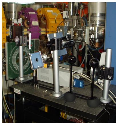
Figure 1: The optical system of the 3+L experiment aligned inside the DAΦNE hall.
