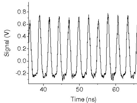
Figure 3: The pattern of the  $e^+$  bunches. The response time of 3+L experimental set-up resolve a separation between consecutive bunches up to 2.7 ns.
