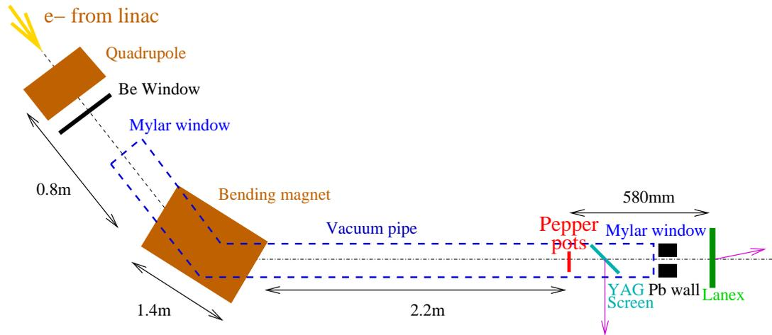
Figure 2: Experimental layout at the DAFNE BTF.
