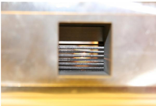
Figure 3: Picture of the sandwich pepper-pot used for our measurement.
