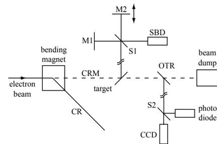
Figure 6: Upgraded CDR setup in the CRM line. A Michelson interferometer, consisting of a beam splitter S1, a fixed and movable mirror, M1 and M2, and a Schottky barrier diode (SBD) detector is installed. Along the OTR optical line a beam splitter S2 is installed, providing a simultaneous beam position and charge reading with the CCD camera and photo diode, respectively.
