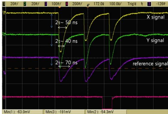
Figure 3: Measured decay time for X signal, Y signal and reference signal, respectively.
