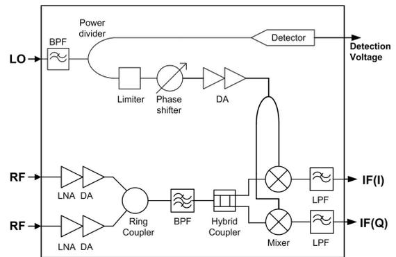
Figure 5: Simplified block diagram.
