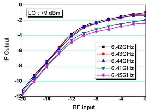
Figure 6: IF output power along RF input power (unit: dBm).
