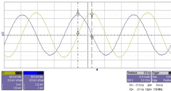
Figure 7: Waveform of output of I/Q measurement.
