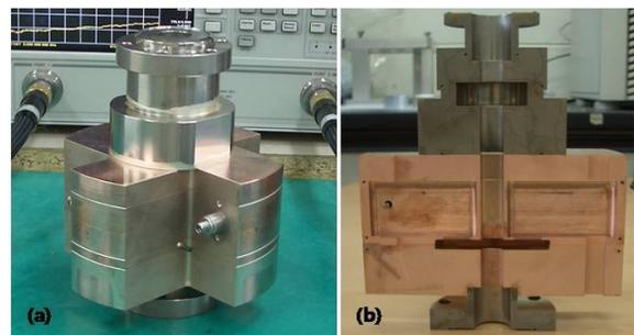
Figure 1: IP-BPM assembled (a), cut for inspection (b).
