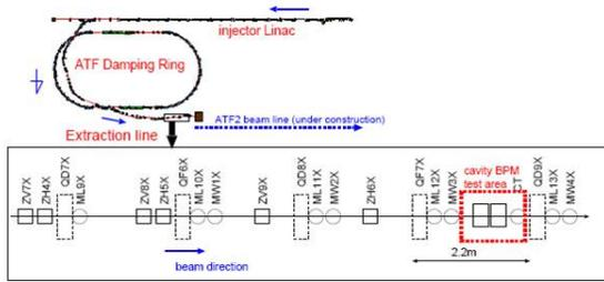
Figure 2: Layout of ATF and ATF2, and the installed position
