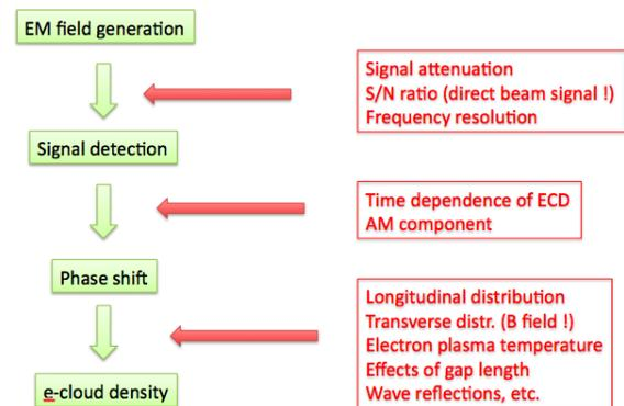
Figure 1: Block diagram of a TE wave measurement procedure, with its sources of error/uncertainty.
