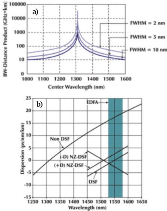
Figure 1: Bandwidth/distance curves for multimode fibers (a). Dispersion curves for single-mode fibers (b).
