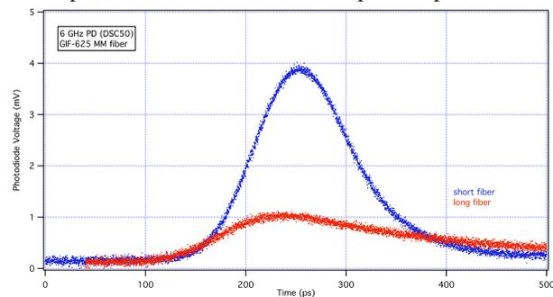
Figure 3: ALS camshaft measurement using the DSC50 photodiode. Short fiber (blue) and 100 m fiber (red).
