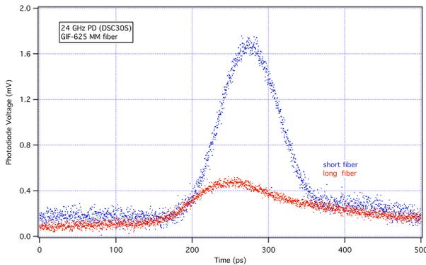
Figure 4: ALS camshaft measurement using the DSC30S photodiode. Short fiber (blue) and 100 m fiber (red).
