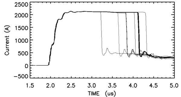
Figure 2 : BPM09 beam current data overlay of 20 shots (#7719-7738). Pulse length is stretched during operations.
