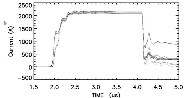
Figure 3: BPM01 through BPM17 beam current overlay for a single shot (#7730).
