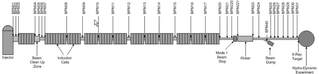
Figure 1: BPM locations as installed on the DARHT II Accelerator.
