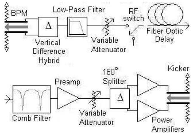
Figure 1: A block diagram of the damping system.
