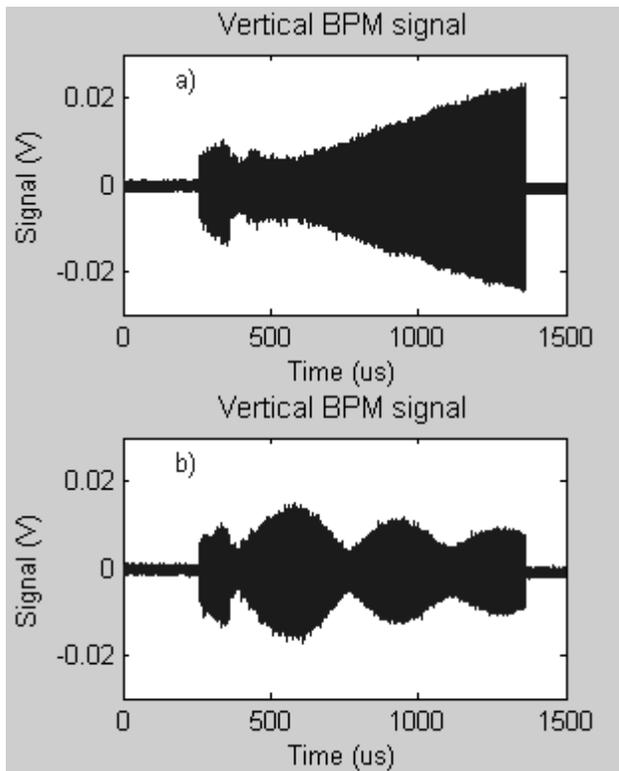
Figure 2: Signals from the wide-band BPM for coasting beam driven transversely at frequencies corresponding to the mode 20 lower sideband (a) and upper sideband (b). These signals are the difference signals from the top and bottom electrodes of the BPM, giving an indication of the vertical position of the beam. The drive was not present as the beam was accumulated during the first 100μs of the signal.
