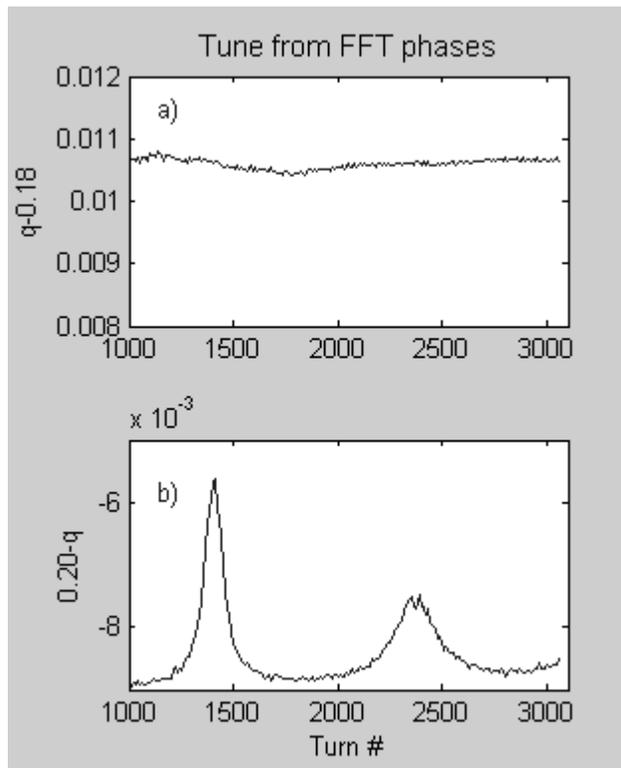
Figure 4: Tunes as determined from the slopes of the phases of Fourier transforms of the data shown in Figure 2. The final 2000 turns are shown. The vertical scales' ranges are the same to allow easy comparison of the magnitudes of variations.
