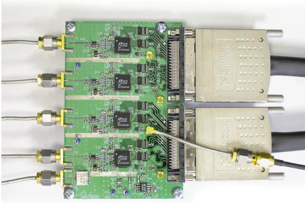
Figure 2: The custom four-channel AFE using Linear Technology LTC2208 ADCs. RF inputs are on the left and connections to the digital I/O cards are on the right.
