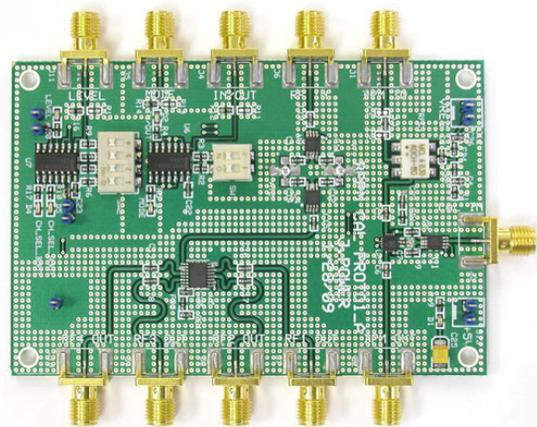
Figure 1: The prototype board with sub-circuits for a single channel of the input module. The circuits include all of the RF switching except for the crosspoint switch.
