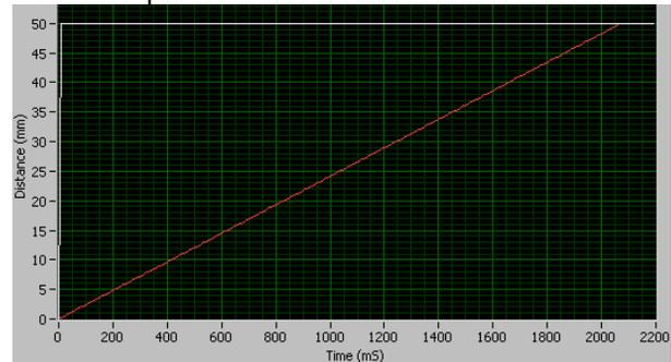
Figure 2: Closed-loop step response, 50-mm move. Setpoint is white, measured position is red.
