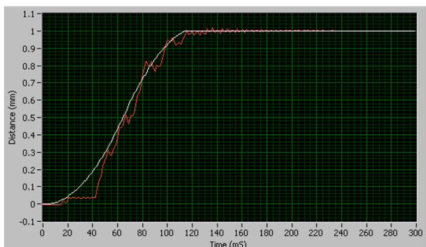
Figure 3: SoftMotion trajectory following, 1mm move. Setpoint is white, measured position is red.
