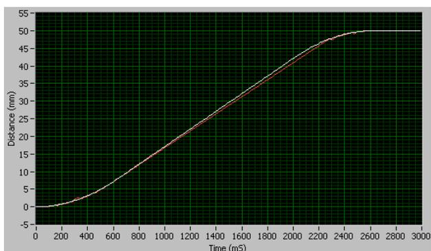
Figure 4: SoftMotion trajectory following, 50mm move. Setpoint is white, measured position is red.
