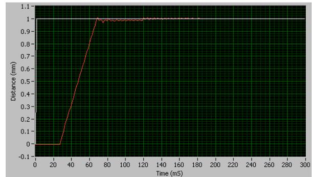
Figure 1: Closed-loop step response, 1mm move. Setpoint is white, measured position is red.
